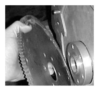
APPLY THREAD LOCKING COMPOUND AND THREAD TO STUDS INTO THE CORRECT HOLES AND USING A STUD DRIVER OR DOUBLE NUTS, INSTALL THE STUDS. WHILE INSTALLING THE TRANSMISSION, REMEMBER THAT THE DOWEL PINS ARE FOR ALIGNMENT ONLY AND WILL NOT BEAR THE WEIGHT OF THE TRANSMISSION.
