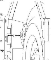
CHECK THAT THE CONVERTER IS SEATED INTO THE FRONT PUMP PRIOR TO INSTALLING THE TRANSMISSION. CHECK THE "PULLBACK" DISTANCE OF THE CONVERTER PRIOR TO INSTALLING THE CONVERTER TO FLEX PLATE BOLTS.
