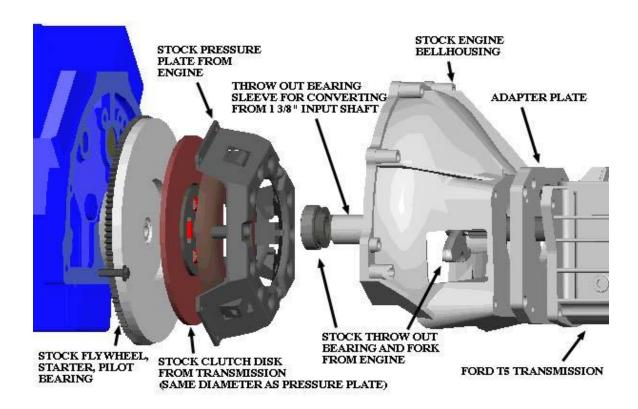
PLACE THE ADAPTER PLATE ONTO THE BELLHOUSING. IF NECESSARY USE A RUBBER MALLET TO FIT THE PLATE UP FLUSH. INSTALL THE SOCKET HEAD CAP SCREWS USING A THREAD LOCKING COMPOUND AND TORQUE. DO NOT USE THE CAP SCREWS TO FORCE THE PLATE ONTO THE BELLHOUSING. MAKE CERTAIN THE ADAPTER PLATE SITS FLUSH TO THE BACK OF THE BELLHOUSING AND THERE IS NO GAP.
