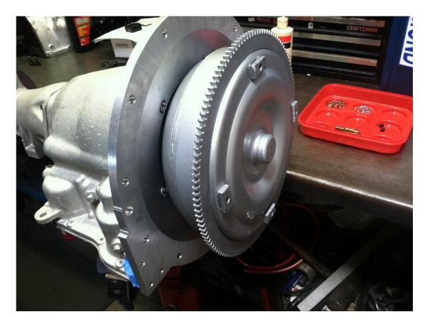
Using the supplied WIlcap instructions, Andy cut the case down and installed the aligned front pump and adapter plate. Wilcap includes instructions on aligning the front pump to the adapter plate or ,as in this case, can perform the service for you.
