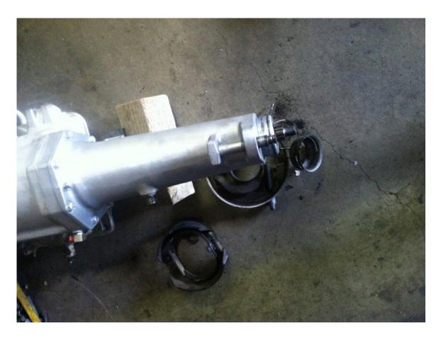
The original Power-Flite has a rear mounted drum parking brake operated by a cable. Andy, having been a MOPAR fanatic forever, knew that many of the Big Block/A-727 motor homes had a similar setup. Using his long list of MOPAR parts suppliers he tracked down the tailhousing, backing plate, drum and other parts needed and with a few modification was able to get the 1970s parking brake hardware onto the back of the new transmission.
