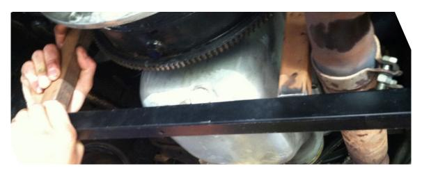
The next step was to get the adapter installed on the new A-727 transmission..
