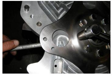
CAREFULLY ALIGN THE HUB SPACER/FLEX PLATE AND THE CRANKSHAFT BOLT HOLES WHILE PLACING THE HUB SPACER ONTO THE CRANKSHAFT. THE HUB SPACER SHOULD BE A CLOSE FIT TO THE CRANKSHAFT. IF USING THE 7/16 NUTS AND BOLTS, THE SLOT CUT IN THE STARTER POCKET IS FOR
