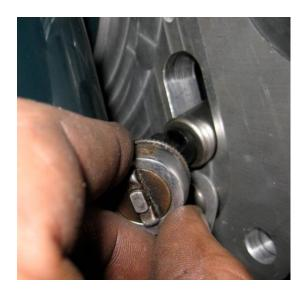
FIT UP THE STARTER MOTOR AND CHECK FOR PROPER RING GEAR TO PINION GEAR ENGAGEMENT. CHECK THAT THE STARTER MOTOR DOES NOT INTERFERE WITH THE HEMI ENGINE BLOCK.
