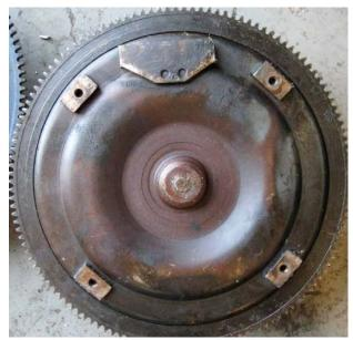
DO NOT USE THE CONVERTER WITH THE BALANCE WEIGHT!! THE CORRECT CONVERTER IS FOR THE 318 C.I. ENGINE.
