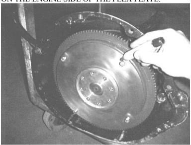
FIT UP THE ADAPTER PLATE TO THE ENGINE BLOCK AND CHECK FOR FIT. THE PLATE SHOULD FIT FLAT TO THE ENGINE BLOCK WITH NO ROCKING OR GAP.
