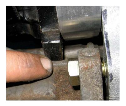
IT MAY BE NESSECARY TO GRIND A SMALL AMOUNT OFF OF THE BLOCK TO ALLOW THE STARTER TO BLOT FLUSH TO THE TRANSMISSION. TORQUE STARTER BOLTS TO PROPER VALUE.
