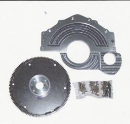
NOTES; The 8BA-350 comes drilled with the Chevrolet Bell housing bolt pattern. On request it can be made with the late Buick, Olds, and Pontiac transmission bolt patterns. The adapter plate can be made with ears that protrude from the sides for use in mounting the engine on request (additional cost). We can supply the starter. Complete instructions are included for installing the adapter.
