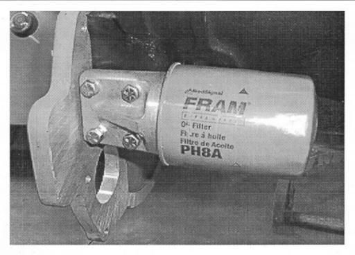
NOTES; The FA1 places the filter in a horizontal position and allows for the starter to be placed on the passenger side. It comes with the gasket and bolts. In some cases it has been found the oil filter adapter block boss was milled shorter on some blocks so it may be necessary to use the smaller oil filter. Complete instructions are included for installing the adapter.
