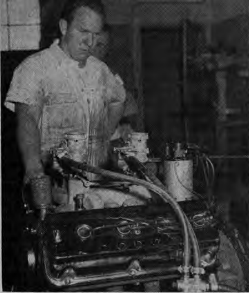
Owner Carl Maginn checks engine over before its run on Wilcap dynamometer. Engine is set up for gasoline, produced 258 bhp.
