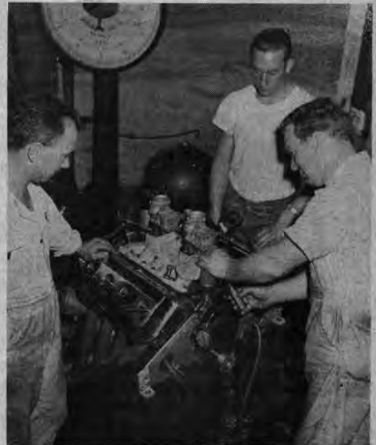
With alcohol fuel and dual carb setup, engine produced 270 horsepower at 5500 rpm.
