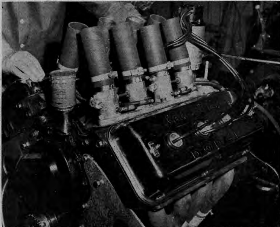
With Hilborn injectors, engine turned up 302 hp on alky. Setup could be used in automobile.
